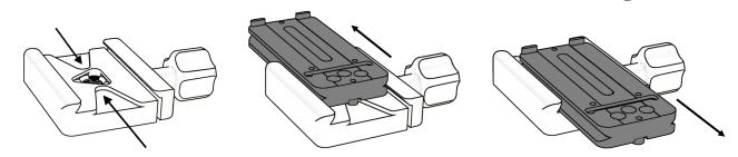
A 3rd Party Clamp Warning: Our safety stop screws work with most 3rd party quick-release clamps, but clamps that do not have channels and are too wide to be straddled by the safety stop screws will not work.
