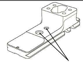
Using the AP-502 without using a quick-release The 3/8 and 1/4 inch holes in the middle section of the plate can be used to attach the foot directly to the threaded stud of a monopod or other lens support equipment, without needing a quick-release clamp.
