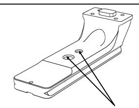
Using the AP-551 without using a quick-release The 3/8 and 1/4 inch holes in the middle section of the plate can be used to attach the foot directly to the threaded stud of a monopod or other lens support equipment, without needing a quick-release clamp.
