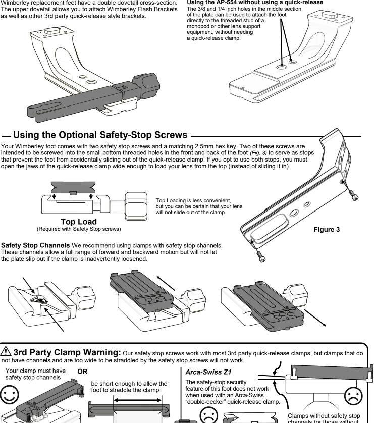
1 3rd Party Clamp Warning: Our safety stop screws work with most 3rd party quick-release clamps, but clamps that do not have channels and are too wide to be straddled by the safety stop screws will not work.
