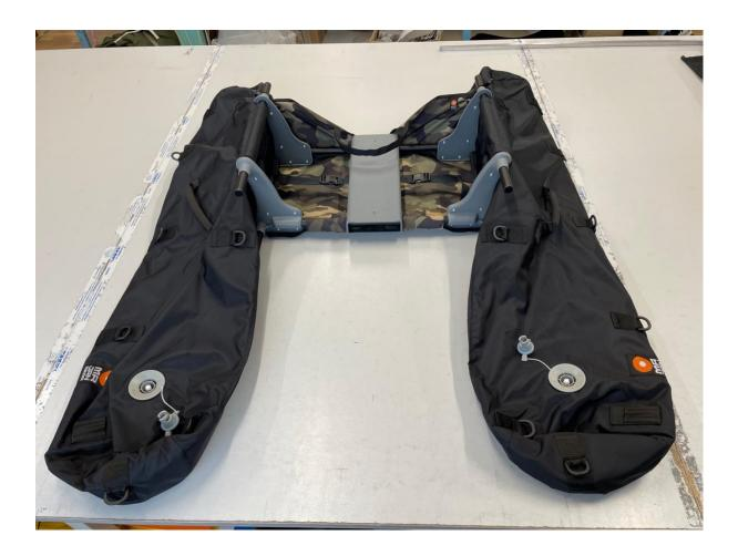
The tent supplied with the FH 3 is easy to assemble – poles in the poles sleeves- position the 4 ends of the poles in the holders on side of the inflated tubes – click the hooks of the tent in the d -rings - - supplied with the tent is a veclro pocket which can be used to keep a spare battery or something else when you are in the water.
