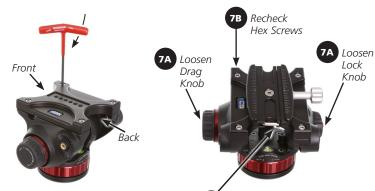
**6.** Take the replacement bridge and re-install the 4 hex screws that were removed in Step 2 with the 4MM hex wrench. Please note: Still keep the Manfrotto Fluid head lock knob and drag knob in the locked position. Make sure that the replacement bridge has the front to the front and the back to the back.
