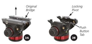
**3.** With the 4 screws removed, gently lift the original Manfrotto bridge and remove as shown in Photo 3 A. After the original bridge is removed, now remove the locking pivot and push button locking tab as shown in Photo 3B. Please note, please keep the original fluid head lock knob and fluid drag knob in the locked position.
